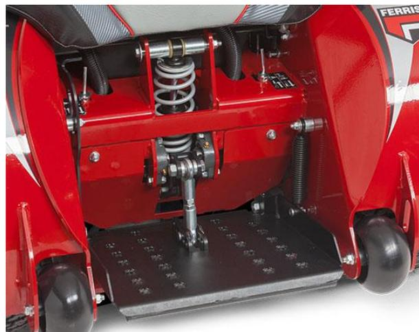
Patent pending suspension platform system, adjustable for large range of weights and operating conditions, optimizing operator comfort.
