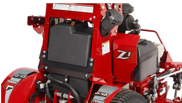
23 Litres fuel tank, centrally located for consistent balance and fuel filler neck conveniently located on the side for easy filling.
