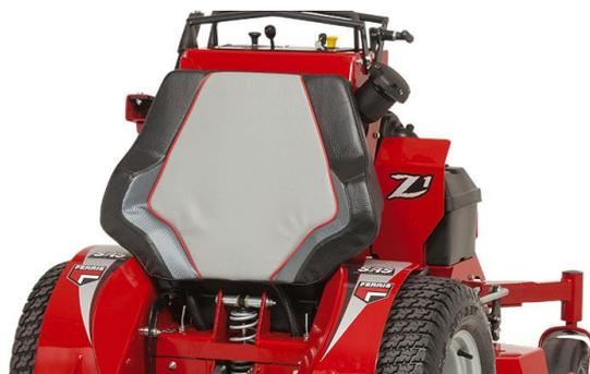
Ergonomically designed thigh pad provides superior operator comfort, especially on uneven terrain.
