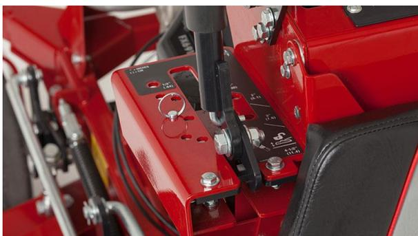
Height of cut is easily changed from operator compartment including transport position for no hassle of curb climbing and trailer loading.
